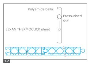
In practice, hailstones with a diameter of 0.79" can reach a terminal velocity of 69ft/s. Under these conditions, traditional roof glazing materials such as glass and acrylic fail.
