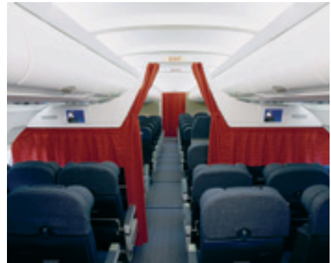
SABIC provided parts made from ULTEM 1668A sheet for the development of Adder cabin dividers.
