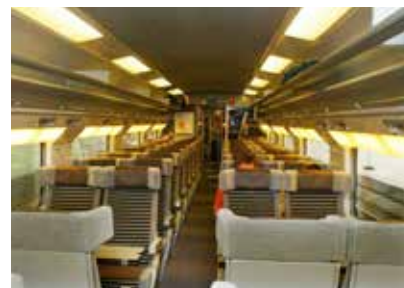
Eurostar international train selected LEXAN sheet for its light diffusers.
