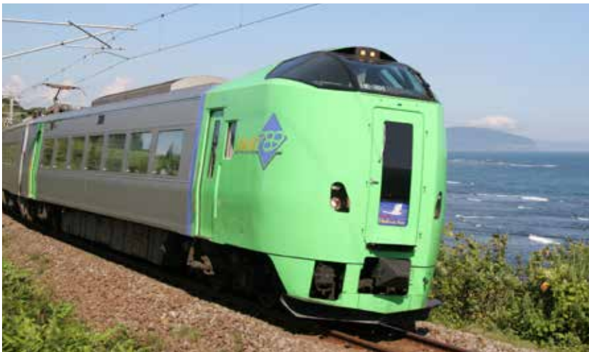
Coated, transparent LEXAN MARGARD Sheet has been chosen by TOHO SHEET & FRAME CO., LTD, a leading Japanese converter, for the double glazing of side windows of The JAPAN RAILWAYS HOKKAIDO.
