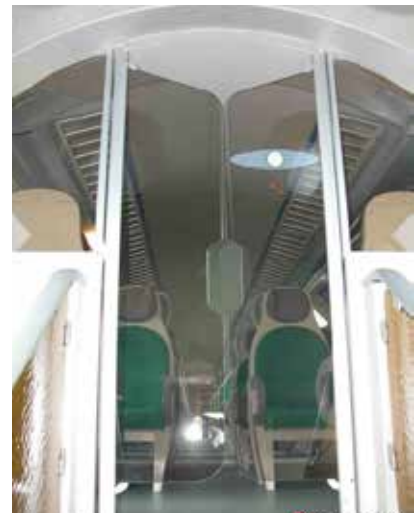
Italian railways compartment separators using LEXAN Margard sheet.
